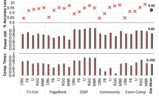
Fig. 8: Normalized GPU completion times, power, and accuracy loss for each benchmark-input combination at the perforation rate pairs (\epsilon_o, \epsilon_i) provided by the learner.
